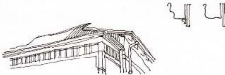
Figure 15.17: Traditional roof plumbing elements include rolled ridge and barge flashings with spear points, ogee or smooth quad gutters and circular downpipes with soldered elbows.
