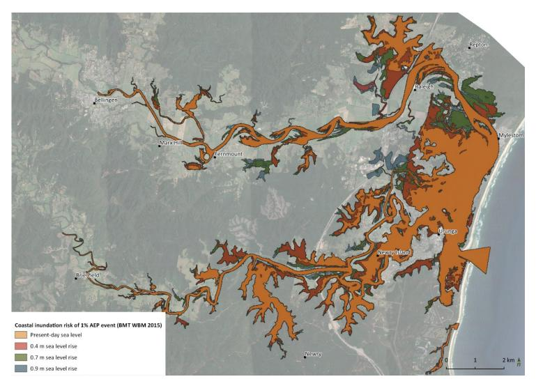
Figure 35. Modelled coastal inundation extents for Bellinger and Kalang River under a 1% AEP event for sea level rise scenarios of present-day, 0.4 m, 0.7 m\* and 0.9 m (BMT WBM 2015).
