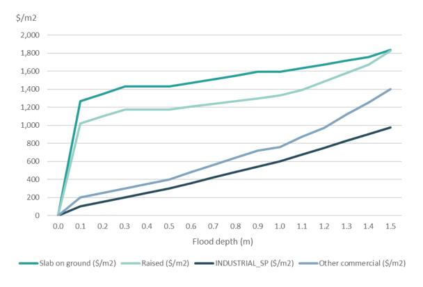
Figure 45. Estimated direct stage-damage curves for buildings (\$/m²)
