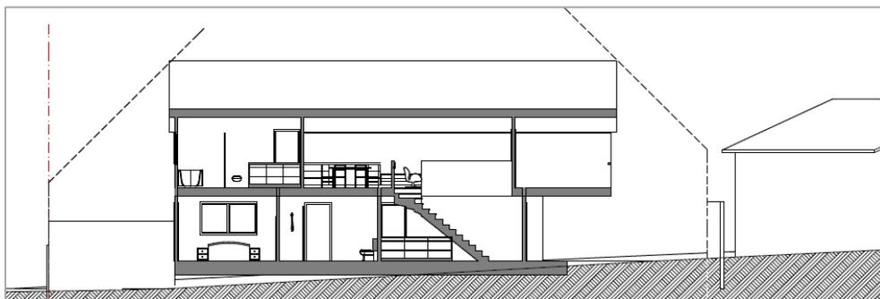
**Section View.** This cross section shows how the design fits within the hypothetical building height plane controls (shown as the black dotted line). The homes measure 7.3m high at the ridgeline, compared to the 5.8m of the existing home.
