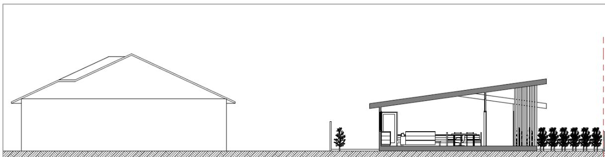
**Section View.** This cross section shows the new home is sensitively designed to be smaller than the existing home. The new home is 4.3m high (compared to 5.8m for the existing dwelling).
