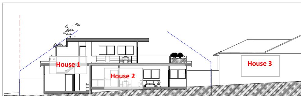
**Section plan.** This cross section shows how the stepped design complies with the building height controls (shown as the blue dotted line). The 6.9m high home is similar in height to the existing home (5.8m).
