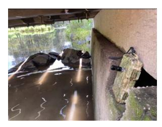
Plate 2.1 Anabat detector positioning (L: Joyces Bridge. R: Justins Bridge)
